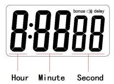
Delay delay indicator: lit indicates that the current delay screen
